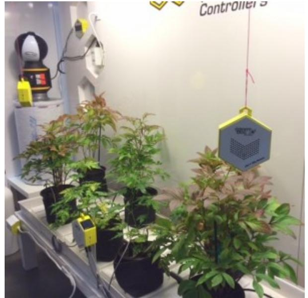
The system uses a variety of sensory devices spread throughout the greenhouse that are capable of measuring key environmental factors like temperature and humidity, along with light and water content.
