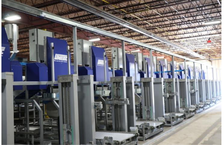
Diamond Fruit Growers' new 18-lane sizer will run 100 bins per hour, replacing two presizing machines
